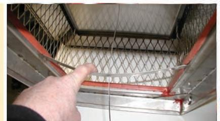
For cleaning, remove the cable guide support by pushing down hard enough so the cable guide support "pops" out of its mounting holes.
