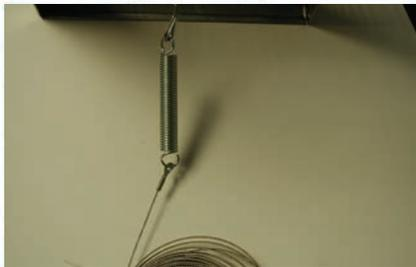
Attach the eyelet end of the 50ft. stainless steel cable to one end of the coil spring of the damper lid cable assembly.
