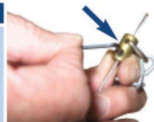
Place in the cable lock at this point and tighten the set screw with the allen wrench. Make all adjustments to the system **before you cut the cable**.
